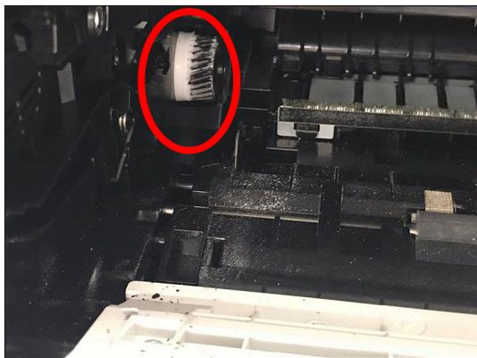
By the end of testing, a significant amount of toner dust had been deposited on the gear of the Brand H machine (above). Several other brands experienced similar build-up on the gears throughout testing.
