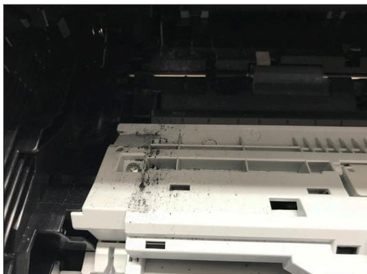
The printer using Brand F cartridges showed significant toner leakage on the manual feed tray, which could contaminate users' hands and pages with toner.
