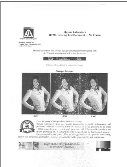
Significant flaking was evident on output from Brand K's fourth cartridge.
