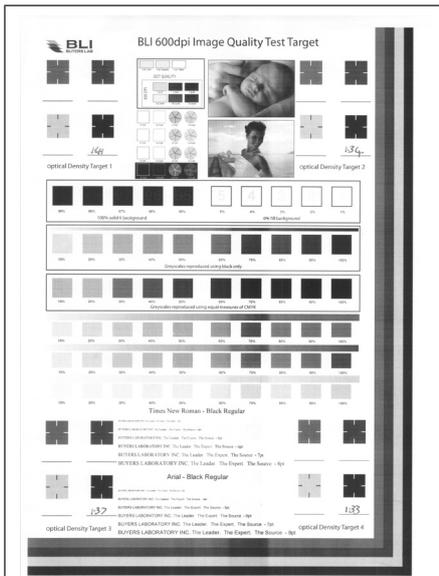
During processing of Brand I's fourth cartridge a dark band appeared in the output, clearly seen at the bottom of the page.
