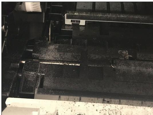
A significant amount of toner dust accumulated in the machine that ran Brand C cartridges (above).
