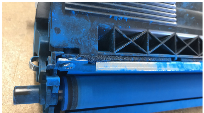
A Brand D cartridge leaked toner inside its packaging.
