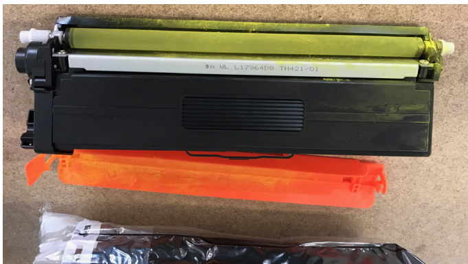
A Brand C cartridge leaked toner inside its packaging.
